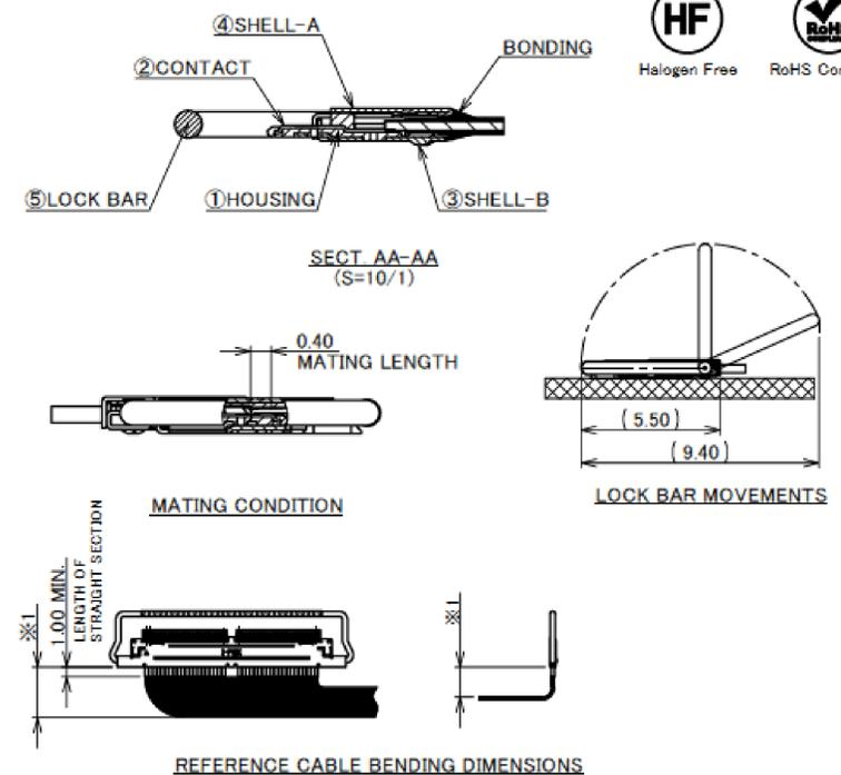
※1: THE BEND DIMENSIONS MAY VARY BASED ON THE SIZE AND QUANTITY OF CABLES. PLEASE CONFIRM THE MINIMUM BENDING RADIUS WITH I-PEX OR THE HARNESS MANUFACTURER.
