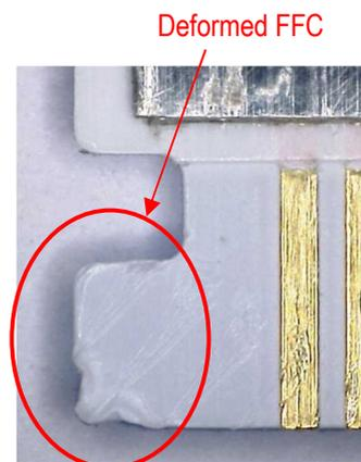
Photo 2-1 Deformed FFC
