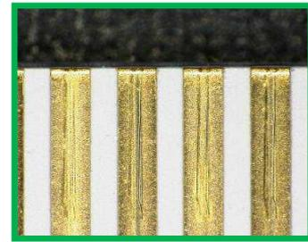
Photo 3-1 (a) Withdrawing FFC/FPC horizontally
