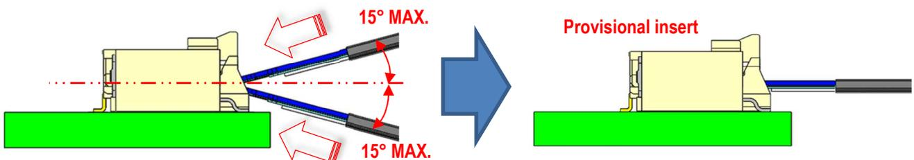
Fig.2-3 FFC/FPC insertion method 3
