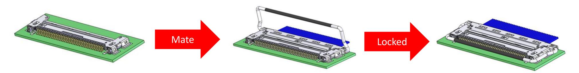
Mechanical locking bar can be locked only when plug is fully mated to receptacle.
