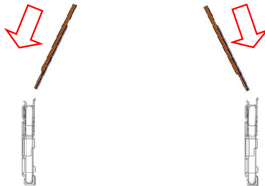
Fig. 6 Incorrect FPC Insertion
