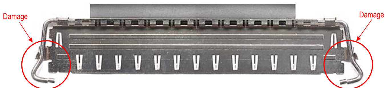
Photo.13 After Deformation Lock Bar Assembly
