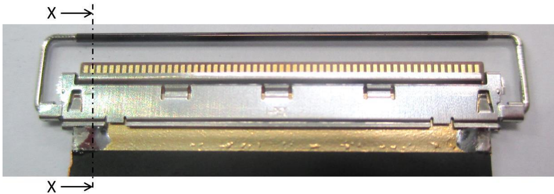
Photo. 3 Soldering of Shell and FPC
